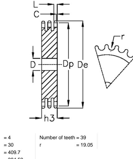
C = 4 D = 30 De = 409.7 Dp = 394.59 For chain size = 1  $1/4 \times 3/4$ For chain type = 20 B-3 h3 = 91 L = 18.2
